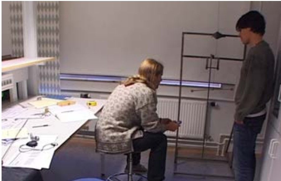
Fig. 2. Photograph taken during the torsion pendulum lab, depicting students observing the oscillations of the pendulum and measuring its period.
