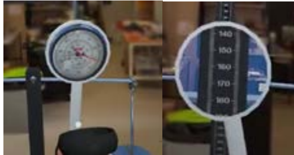
Fig. 3. In headset image of the magnifying glass effect on a gauge (Left) and ruler (Right).
