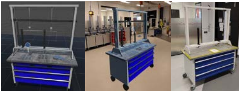
Fig. 4. 3D Unity scene view with the model of the experimental apparatus (left), In AR headset view of apparatus in the lab (center) and the real unit in the same lab (right).
