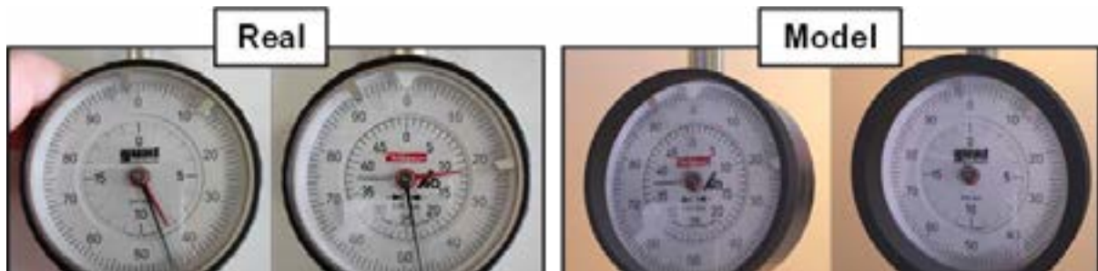
Fig. 2. Photo of actual dial gauges (Left), Texture mapped glTF 3D model (Right).
